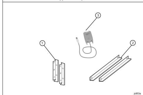
Option **Item Part Description** Number Number 1 1CM Rack Mount Flange Kit (For use without handles) 2 Rack Mount Rail Set 1 1CP Rack Mount Flange Kit (For use with handles) 2 Rack Mount Rail Set 3 82375A USB/GPIB Interface (included with Option 083 only)
